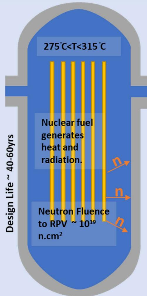
Figure 1: Simplified schematic of water-cooled reactor pressure vessel giving key points on design life and environmental conditions endured by RPV steel. Lifetime, fluence and temperature range acquired from [2].
