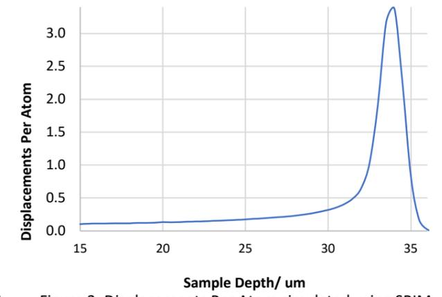
Figure 2: Displacements Per Atom simulated using SRIM for 2.9MeV protons incident on FeMnNiSi model alloy.
