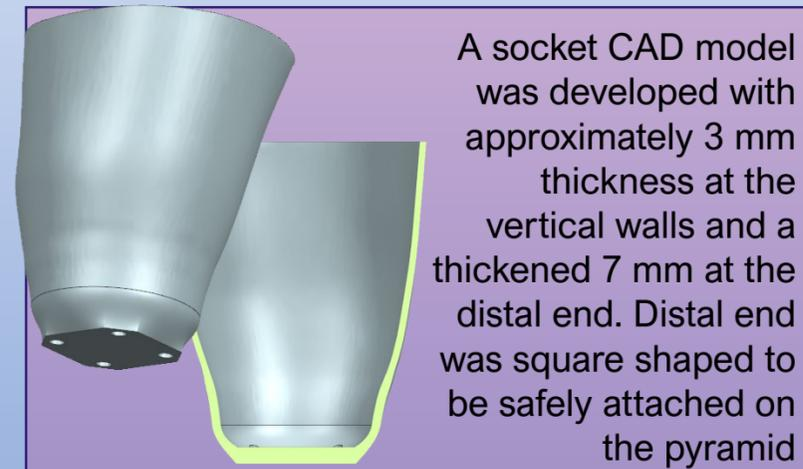
A socket CAD model was developed with approximately 3 mm thickness at the vertical walls and a thickened 7 mm at the distal end. Distal end was square shaped to be safely attached on the pyramid
