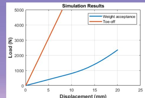
Results from Condition I indicate that the socket can withstand approximately 5000 N without failing easily surpassing 3890 N that was the required level.
